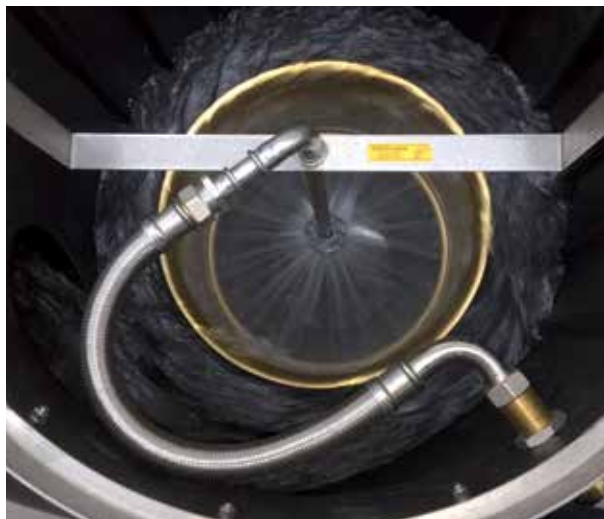
Cleaning nozzle for Vortex Finefilter WFF 300
